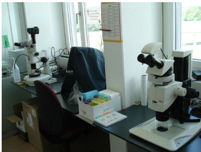
Fig. S1. Two working spaces equipped with high-end stereomicroscopes and cameras. Microscopes are equipped with dark field illumination. Note: for working on the microscopes, blinds of the windows would be lowered to avoid reflections and uncontrolled illumination. Next to the microscopes, a calendar is given to reserve slots for individual work-projects. Photo by Florian Altermatt.
