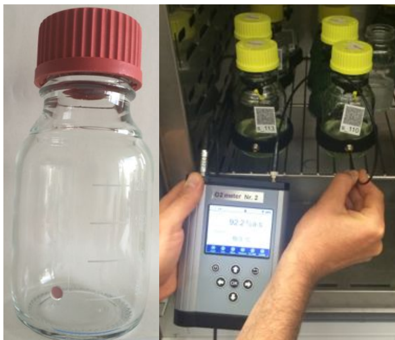
Fig. S3. Left: A sensor (optode by PreSens GmbH) glued to the inner surface of a standard culture vessel. Right: A measurement of oxygen saturation being made. Microcosms are fitted with a guide to ensure the fibre optic cable is correctly placed. Photos by Owen Petchey.
