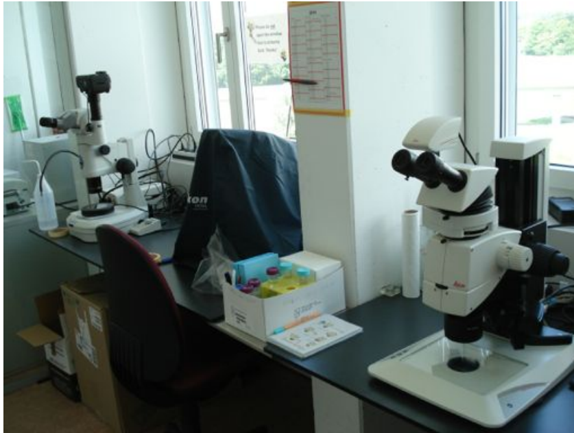
Fig. S5. Two working spaces equipped with zoom stereomicroscopes and cameras. Microscopes are equipped with dark field illumination. Note: for working on the microscopes, blinds of the windows would be lowered to avoid reflections and uncontrolled illumination. Next to the microscopes, a calendar is given to reserve slots for individual work-projects. Photo by Florian Altermatt.
