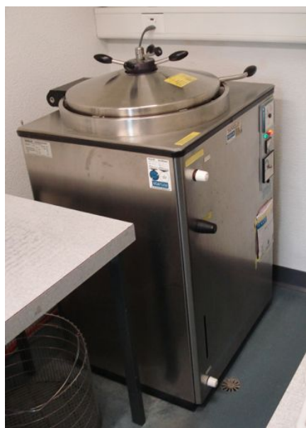
Fig. S2. Autoclave used to sterilize protist medium and equipment used for protist experiments. Photo by Florian Altermatt.
