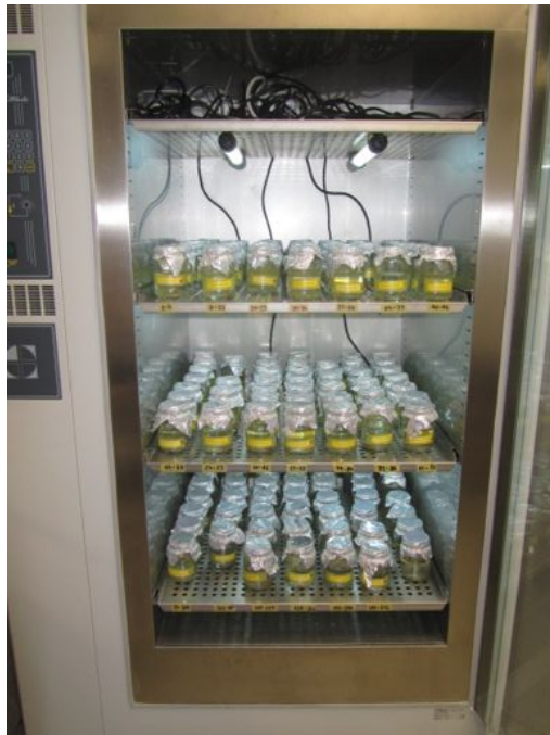
Fig. S3. Example of an incubator with individual protist microcosms (showing the experiment by Mächler & Altermatt 2012). The incubator is temperature-controlled (20 °C) and has constant fluorescent lighting. The position of the replicates of each treatment is randomized across the incubator to avoid biases due to position in the incubator. Photo by Elvira Mächler.
