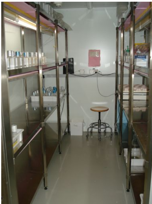
Fig. S4. Temperature controlled walk-in chambers in which protist experiments can be conducted. At each shelf, homogeneous light-sources are installed (note the insulation above each light to avoid warming of the shelf above it). Photo by Florian Altermatt.
